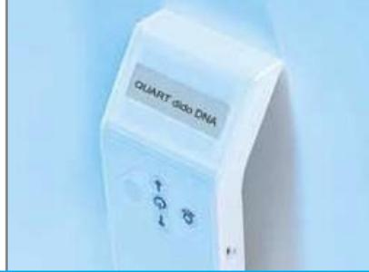
The QUART dido DNA system is a special development oriented to a specific task; it serves to show the dose delivered in an x-ray system right after the exposure. It is derived from the established diagnostic QUART measurement solutions for conventional dosimetry.
