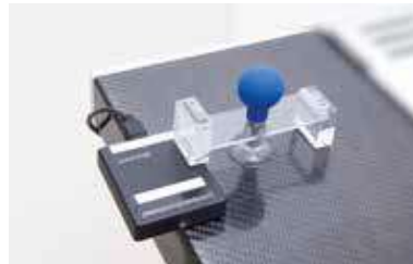
QUART nonius with bridge holder ready for measurement at a mammography system
