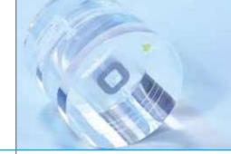
The QUART DVT\_AP phantom is designed to be used as a technical tool for QA/QC testing in Cone Beam CT (CBCT), Dental Volume Tomography (DVT) and DICOM based 3D Imaging applications.
