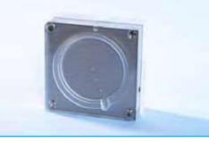
The QUART dent/digitest phantom is designed to be used for QA/QC routine testing in Dental X-Ray applications ranging from intra-oral, panoramic and cephalometric equipment.
