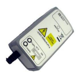
The power element is basically made up of a power relay which is switched by the actuator output (or straight from the central unit). The connection is by cable – the contacts of the actuator's memory relay switch voltage on the power relay coil. The power element must be connected to the distribution network voltage, so it will mostly be located near an actuating unit (fan, recuperation unit, etc.)..
