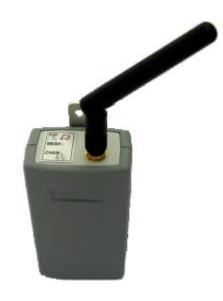
The repeater is an element designed to increase the system range, i.e. connection between the central unit and other elements (probe, actuator) where the signal is weak at direct connection. This may happen in a free space at a too long distance. The range in buildings depends particularly on the building material (walls, partitions, floors, etc.). For example, in the case of a reinforced concrete skeleton, which represents efficient shielding, a problem can occur even at very short distances.
