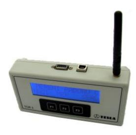
The central unit controls the operation of the radon concentration measuring and control network. It collects data from individual elements (probes), it operates actuating units and via the central unit the network is configured and all parameters are set.
